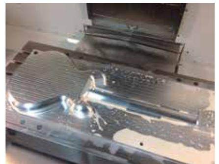
Profiling the resonator plate in the VMC.
